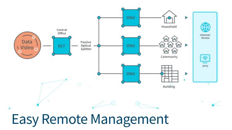
GP601GVR support the ONT Management and Contol Interface (OMCI), making it easy to configure, activate and manage remotely from an Optical Line Terminal(OLT).
